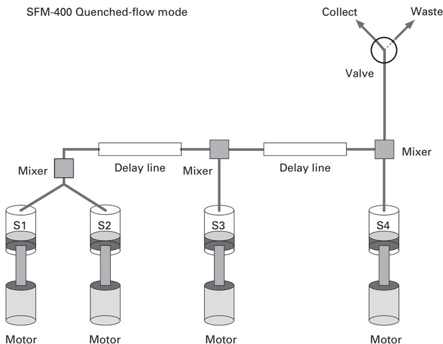
Fig. 15.12 The BioLogic stopped-flow and quenched-flow apparatus. The reactants are placed in separate syringes each driven by a microprocessor-controlled stepping motor capable of delivering  $0.01$  to  $10.00 \text{ cm}^3 \text{ min}^{-1}$  with a minimum injection volume of  $10\text{--}30 \text{ mm}^3$ . The reactants are pre-mixed before they
